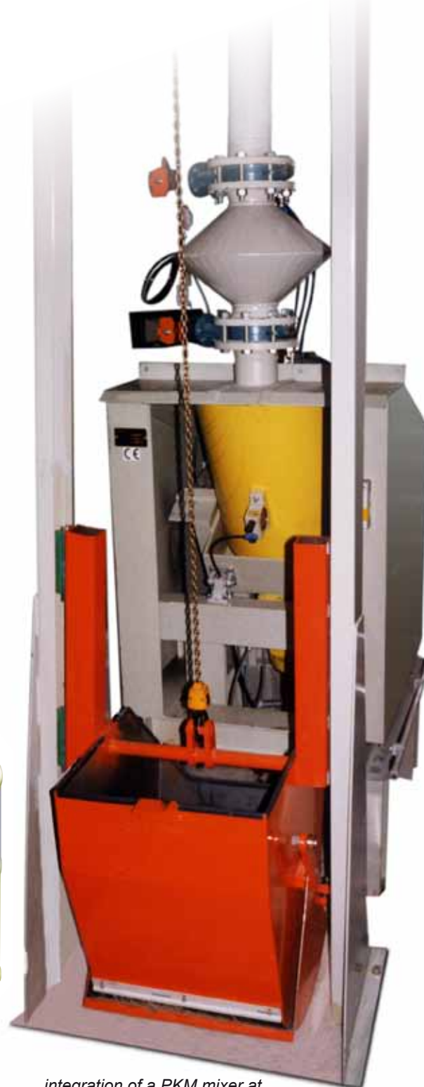
integration of a PKM mixer at floor level with a HLK sand distribution system
